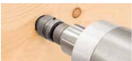
5. Countersink WB directly with insertion sleeve.
