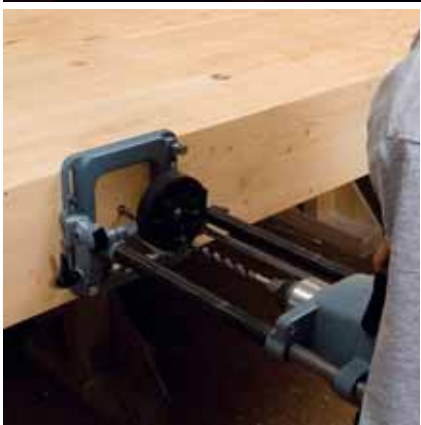
1. Pilot drilling with column type drill.
