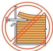
Nail at wrong angle Do not bend tab back
